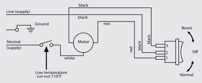
Fig.4 Wiring diagram
