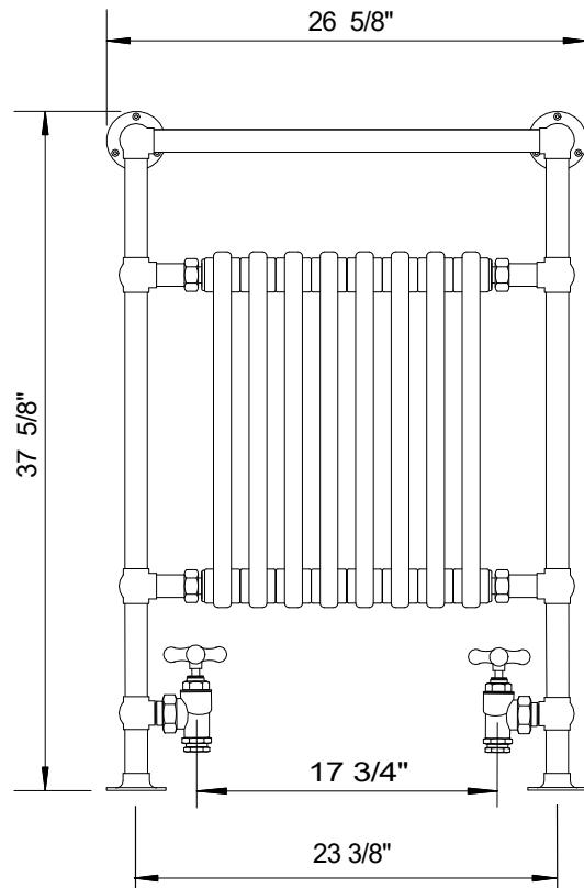
**NOTE:** Valve rough-in centers may vary from 18½" - 19" depending on valve spud insertion depth.
